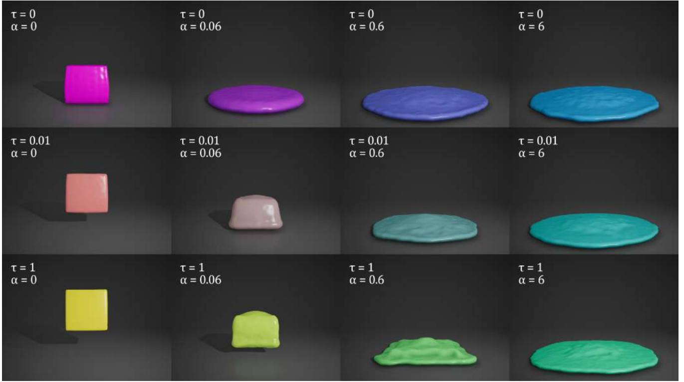
Fig. 4. Viscoelastic cubes are dropped on the ground. By varying two physics-based parameters, the conformation relaxation time constant \tau and the compliance \alpha , we achieve materials that bounce elastically (yellow), appear highly viscous (magenta), or splash as an inviscid liquid (cyan).
