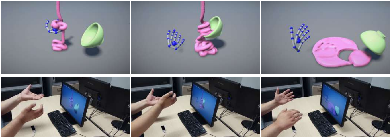
Fig. 10. Three screen captures of interactive manipulation of a viscoelastic fluid, consisting of up to 15k particles, and simulated at 30 ms/frame. The motion of the hands is tracked using a Leap Motion™ device, and this motion is applied to a virtual hand and a bowl, which interact with the coiling fluid. We also demonstrate interactive changes to material parameters.
