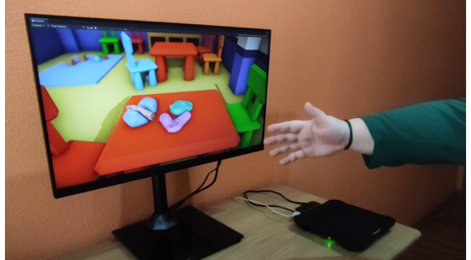
Fig. 1. Arts & crafts in the virtual classroom. We introduce a novel model of clay that allows interactive and highly realistic deformations, merging, and splitting. We also introduce an ultrasound rendering algorithm that enables a tangible interactive experience.
