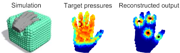
Fig. 3. Our tactile rendering algorithm proceeds according to these steps, from left to right: (i) The particle-based simulation computes forces and deformation on clay particles due to the interaction with ghost particles on the hand (Section III). (ii) We compute a pressure field on the ghost particles on the hand (Section IV-A). (iii) We compute the location and pressure of focal points such that the reconstructed pressure field is optimal, and these focal points are commanded to an ultrasound array for amplitude-modulation rendering (Section IV-B).
