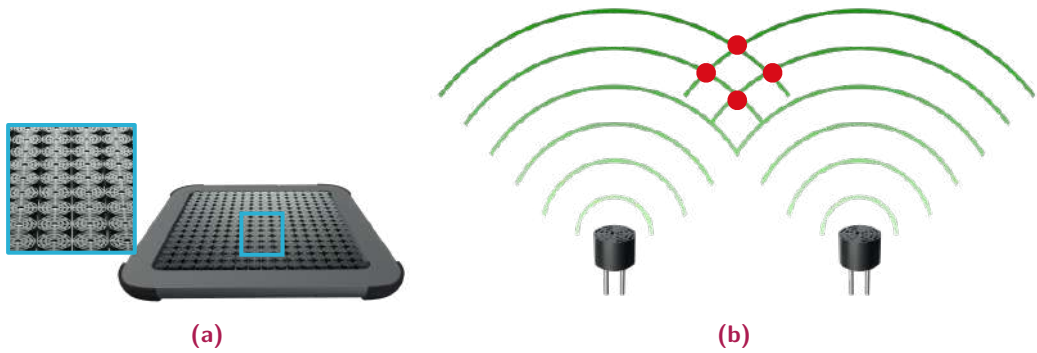
Fig. 2.11.: (a) Illustration of a ultrasonic phased array board modelled after the Ultraleap STRATOS Explore (USX). (b) Transducer activation is modulated to achieve maximal pressure intensity at desired locations in space.
