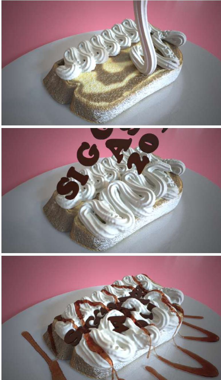
Fig. 3.1.: A complex multiphysics simulation involving viscoelastic fluids, rigid bodies, and deformable bodies. We simulate whipped cream and strawberry syrup efficiently using our novel viscoelasticity model based on conformation constraints. The complete scene consists of 150,000 particles and runs at 1.13 seconds per frame.
